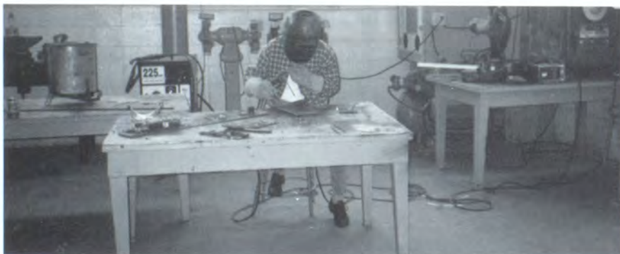
Practicing welding a piece of mild steel in Mr. Ellison's technology class, is Miranda Taylor. She is using an electrode to develop an arc
