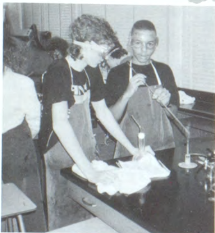
Juniors Andy Lortz and Bryan Fuel fire polish the end of a glass tube for their wash bottle. The wash bottles made in the first lab were used to clean beakers and flasks.
