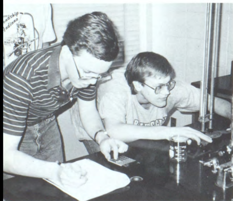
Matt Smith reads the height of mercury in a J-tube while Gary Gick records data. They used the J-tube to determine the air pressure.
