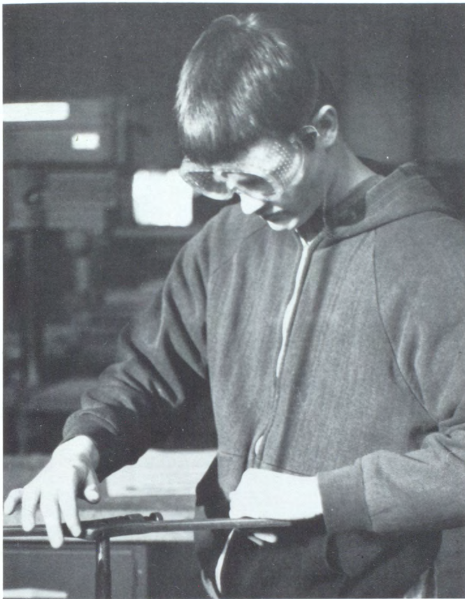
Senior Tony Sullivan is putting threads on a bolt with thread die. The bolt was previously made on a metal lathe.
