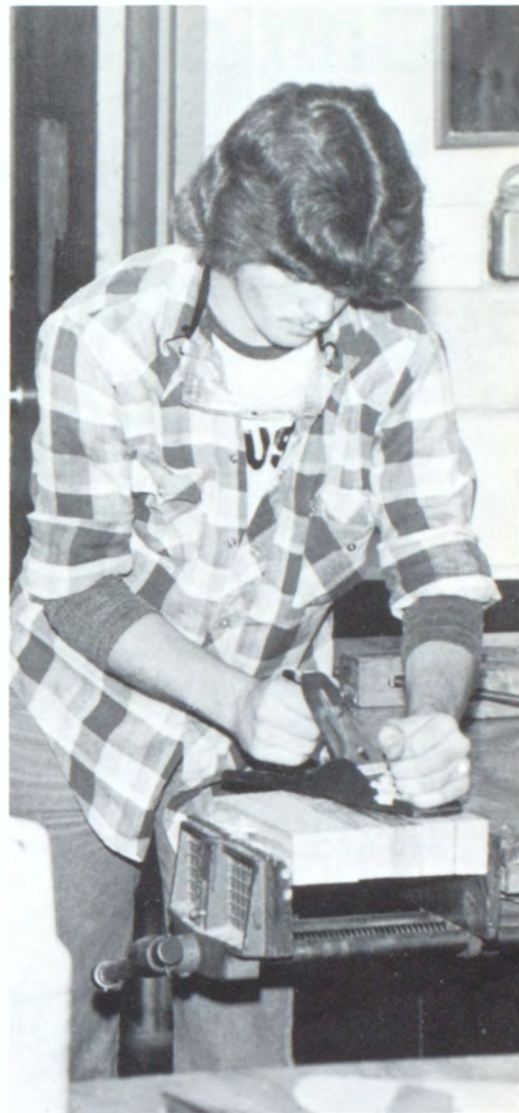
Using a vise to hold the wood allows Steve Watkins to work a hand plane with more ease.
