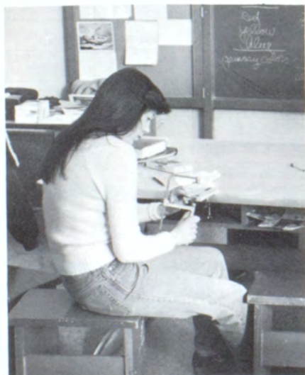
Julie Essex, a member of the Metalsmithing class, pierces her pendant with a design. Doing this required a jeweler's saw frame, numerous saw blades and a large amount of patience.
