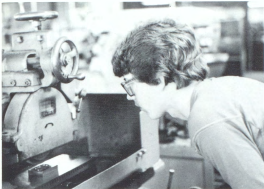
Joe Coy flattens out the top of a half-inch piece of steel which is part of the process of making a name plate in the shop area of his Blue River class.
