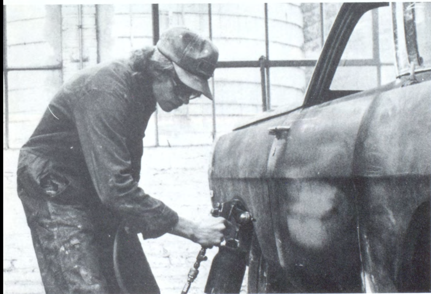
Charlie Moore, clad in overalls, uses a spray gun to prime a car, readying it for painting.
